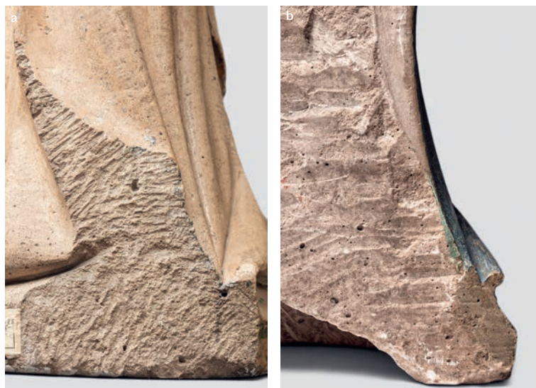
11 The Madonna of Hallstatt (a) and the Madonna of Bad Aussee (b), details of the surface of the cast stone with visible bubbles, view of the backs.
