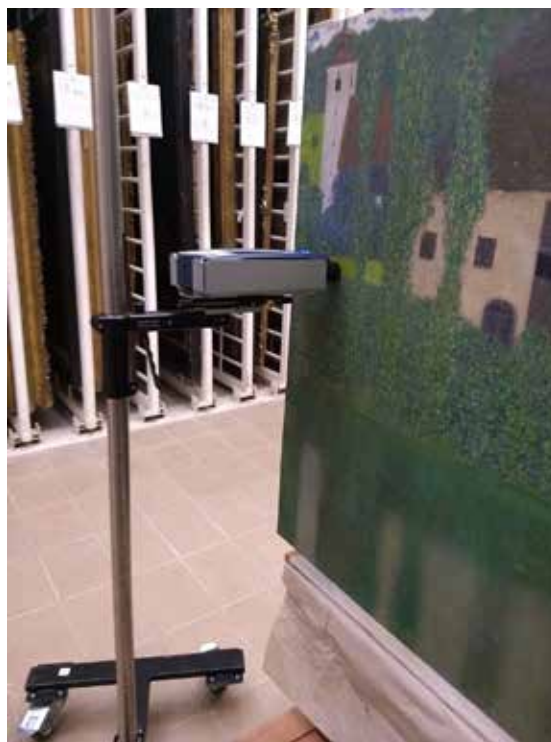
4 Measuring with a Raman spectrometer equipped with a duo laser operating at 780–1064 nm.
