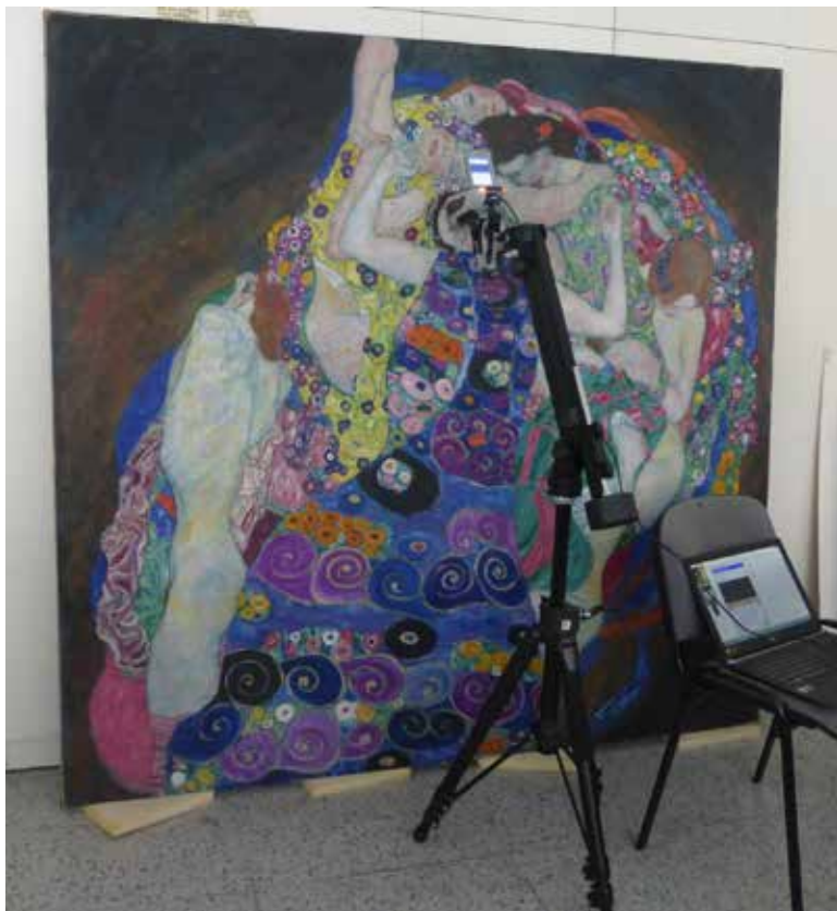
1 Examination of the Virgin with a portable XRF spectrometer.
